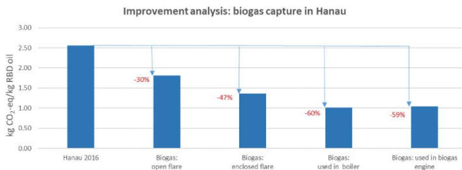
**Fig. 14.** Reduction of GHG emissions for 1 kg of RBD palm oil production achievable by implementing four different biogas treatment options in Hanau POM: biogas capture with open or enclosed flaring and utilization in boilers or biogas engine. The Hanau's baseline scenario, 'Hanau 2016', does not include any biogas capture facility, because POME are currently treated in an open pond system.
