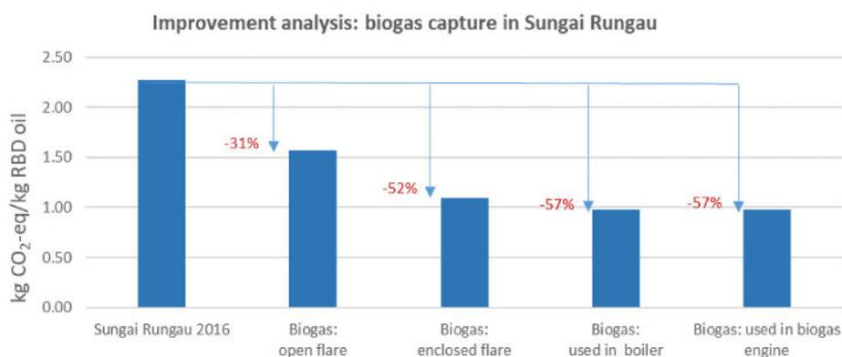
**Fig. 15.** Reduction of GHG emissions for 1 kg of RBD palm oil production achievable by implementing four different biogas treatment options: biogas capture with open or enclosed flaring, and biogas capture and utilization in boilers or biogas engine. The Sungai Rungau's baseline scenario, 'PT SMART 2016'. Does not include any biogas capture facility, because POME are currently treated in an open pond system.
